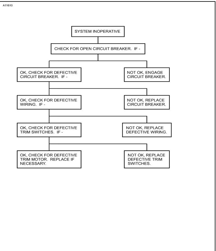
Figure 101 : Sheet 1 : Electric Elevator Trim System Troubleshooting Chart
